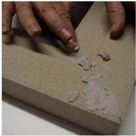
Thumb in resin to seal gaps - take care to check the entire moulding surface
